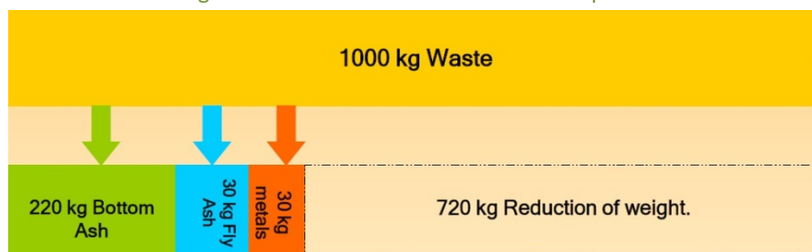
Figure 3. Mass balance of an incineration plant.
